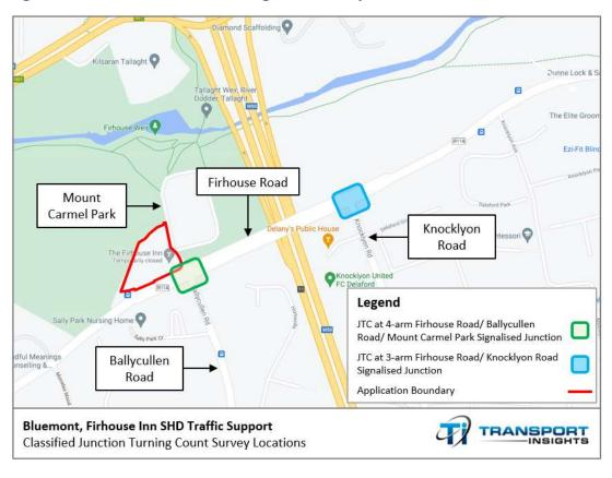
Figure 4.1 Classified Junction Turning Count Survey Locations
